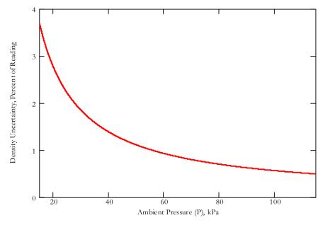
The plots show the uncertainty in the density increases significantly for low temperature and ambient pressure. For this example, at standard ambient conditions, the density uncertainty is about 0.6% of reading.
