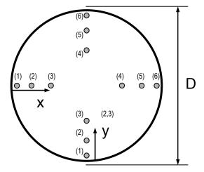
D is the duct diameter, N is the number of points along the diameter, and i is the location of the measurement point (N=6 as shown on the figure). Commonly used Tables are given below:
